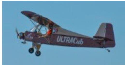
The UltraCUB is a derivative of the Kitfox Lite, by James Weibe of Belite Aircraft. It has the full span flaperons of the Kitfox series, and folding wings. This was one of the first models intended to use a 4 stroke ½ VW engine. It is of aluminum construction and is put together with pulled rivets.
