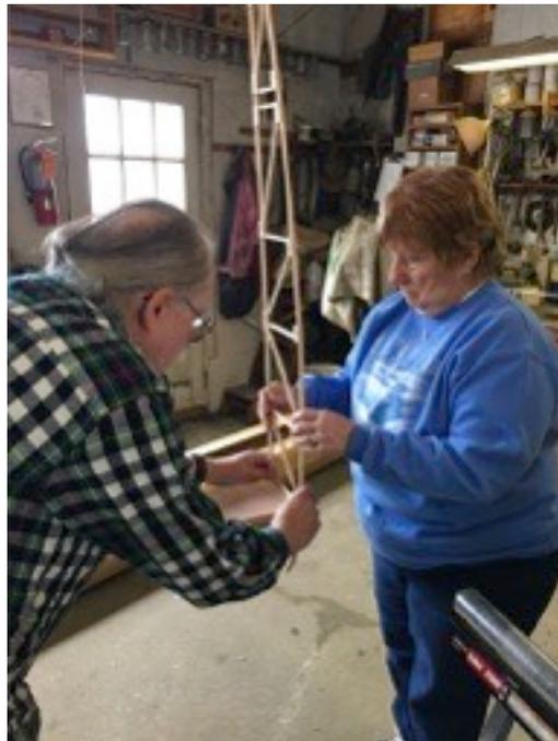
Vet and Gail test fit a wing rib to a spar. Tight and snug like it should be.
