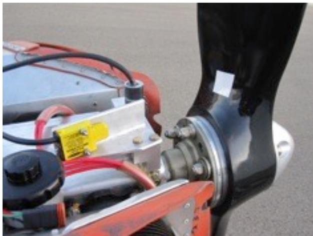
An accelerometer measures the force of vibration. It must be rigidly mounted to the engine and oriented to point in towards the crankshaft. The photo-eye reads a small piece of reflective tape attached to a prop blade. The position of the photo-eye defines the "Zero Reference Point." The control unit knows
