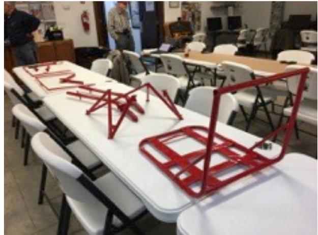
The big news on the metal front is that everything EXCEPT the fuselage has been primed and/or painted. Primed but unpainted pieces (tail feathers and landing gear) will be covered in fabric. The struts, the seat and control stick, the engine mount, and other parts of the landing gear are all now shiny RED!
