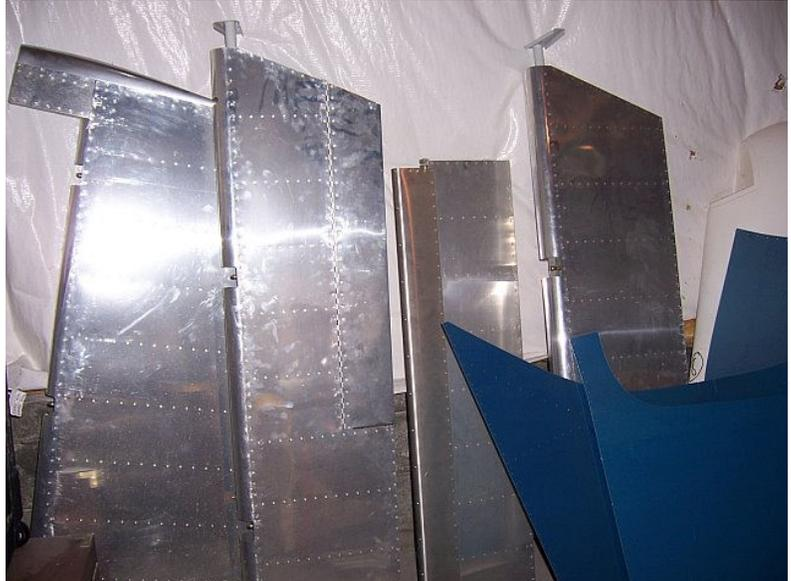
Left to right: Rudder, elevator, aileron, elevator.
