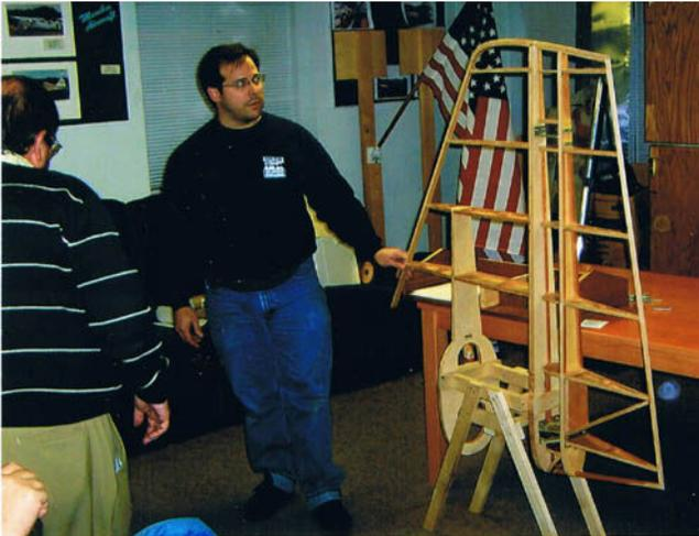
Jarrel Battaglia displays his rudder with the hinges attached. It would be a shame to cover it.
