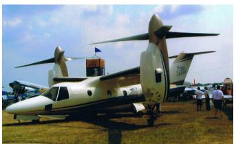
I really want to see one of these fly. This is a Bell/Agusta BA 609 Tilt Rotor. It can seat 12, flies at 275 knots, ceiling of 25,000 feet, and a range of 700 nm.
