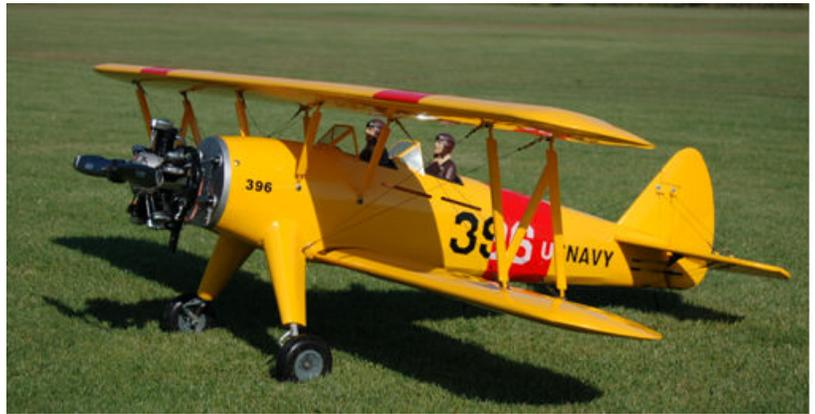
Just under ¼ scale Stearman with 5 cylinder radial engine
