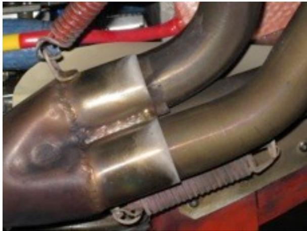
The three stub pipes are welded together such that there is no way to fit clamps on the individual pipes, and their alignment with header pipes is less than ideal, so clearance is needed to assemble the things. Also a builder needs to maintain some float to account for thermal expansion.
