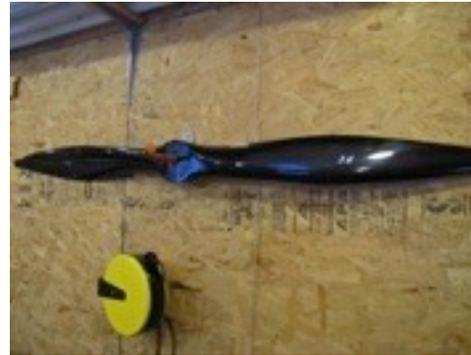
Notice that it also has a similar shape. This design is also intended to account for many factors, such as the torque of my engine, and the speed of the Kitfox (slow), and again producing the ideal distribution of lift along the blade for my own aircraft and engine. This is an experimental design, and flight testing will determine whether or not we have it right.
