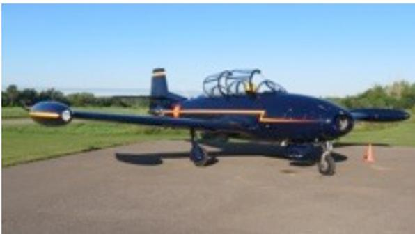
It is capable of flying 430 MPH at 23,000 ft., ceiling is 42,650 ft., range of 930 miles. It has underwing hardpoints for a variety of weapons with a 22-mm cannon in the nose. Imagine saying that about YOUR airplane! Source: <[warbirdalley.com/saeta.htm](http://warbirdalley.com/saeta.htm)>.
