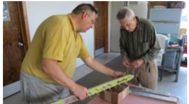
Jack Frenz spent a day working on the Onex. He drilled, cleco'd, riveted, and signed his name on the vertical stabilizer.
