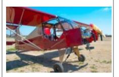
KitFox Lite derivative by James Weibe of Belite Aircraft, Full-span flaperons, folding wings, 4-stroke 1/2 VW engine.
